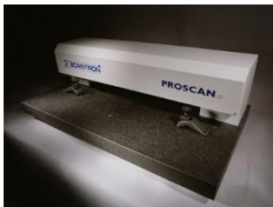
Surface roughness and flatness analysis
