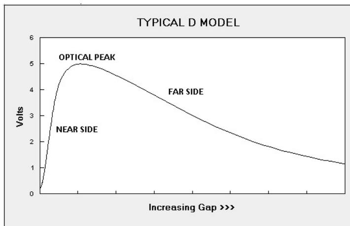
The output function includes a region of maximum output voltage referred to as the OPTICAL PEAK. The useable operating range of these devices includes linear ranges on both sides of the peak, as well as operation at the peak itself. Operation in the NEAR SIDE region gives high sensitivity with limited operating range. Operation on the FAR SIDE gives moderate sensitivity with greater operating range. Operation at the Optical Peak has zero displacement sensitivity, but is reflectance dependent.
