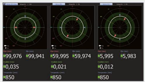
LARGE DISPLAY OF THREE MEASUREMENT FRAMES IN ONE PRODUCTION LINE. SHOWS PROFILE GEOMETRY WITH TOLERANCE FIELDS AS WELL AS MOST IMPORTANT MEASUREMENT VALUES FOR EACH FRAME.
